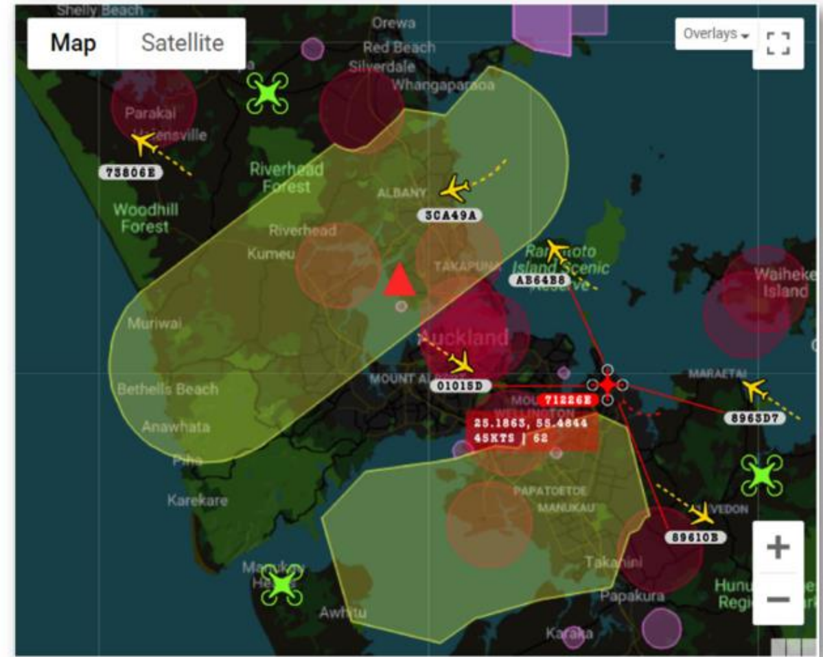
Auckland area showing aircraft, approved UAV flights (green UAV), one approved UAV who has deviated from their flight path (red UAV), and one non-cooperative drone (RED triangle)
